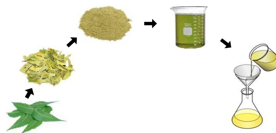
Figure 2: Dye Extraction Process from Neem Leaf.
